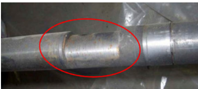
Shaft damage at bearing location
