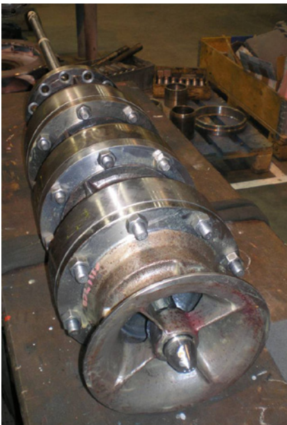
Inspection of the upgraded rotor 18 months after operation
