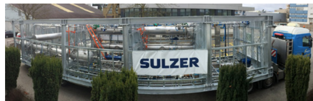
Integrated phenol recovery plant in a skid module
